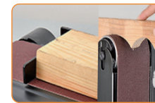
Driven Drum sanding 从动滚筒打磨
